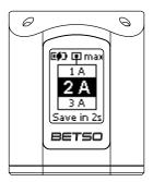
Customizing the charging process to suit your preferences is simple with the SB CHARGER's adjustable maximum current flow settings. The maximum current flow determines the rate at which your smart batteries charge. Selecting the appropriate current flow setting optimizes charging efficiency for your specific requirements.
