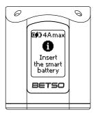
If the battery is not detected when the charger is turned on or if the user disconnects the battery, the display changes to the "Unplugged battery" screen. This screen shows a visual notification in the form of the symbol "i," prompting the users to insert the smart battery.
