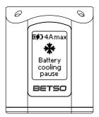
The battery cooling pause screen on the SB CHARGER plays a crucial role in managing and optimizing the charging process. When the temperature of the charging battery reaches the maximum limit, the battery cooling function intervenes, and a cooling alert is displayed.
