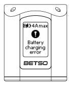
If the error is caused by the connected battery, the screen displays an exclamation mark symbol, accompanied by the message "Battery Charging Error." This visual alert indicates that there is an issue with the smart battery or the power supply, prompting users to investigate and resolve the problem.
