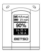
The main screens of the SB CHARGER provide a comprehensive overview of charging information, ensuring users have real-time insights into the charging process. Each screen features five lines displaying key charging metrics. The last two lines (Screen "A" and Screen "B") alternate continuously at an interval of 1.5 seconds:
