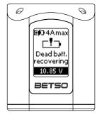
When a dead battery is detected, the recovery process starts automatically. This is indicated by a screen with an exclamation mark in the battery and the text "Dead battery recovering". SB CHARGER will charge the battery first with a small current. When the battery reaches a healthy level, it will start charging at full speed. At the bottom of the screen, the charging current and voltage information periodically alternates.
