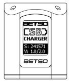
After connecting the power adapter to the SB CHARGER, a startup screen will display the BETSO logo, device name, serial number, and hardware/firmware version. This screen can also be accessed by pressing and holding the button for more than 5 seconds, which resets the device's microcontroller. For detailed information, refer to Chapter 7.11 System.
